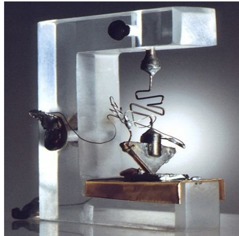
First Point Contact Transistor of Bardeen and Brattain
